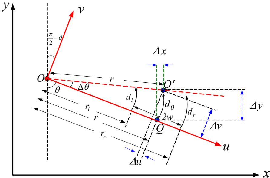
Fig. 2. Rotational dynamics of a holonomic AGV.
