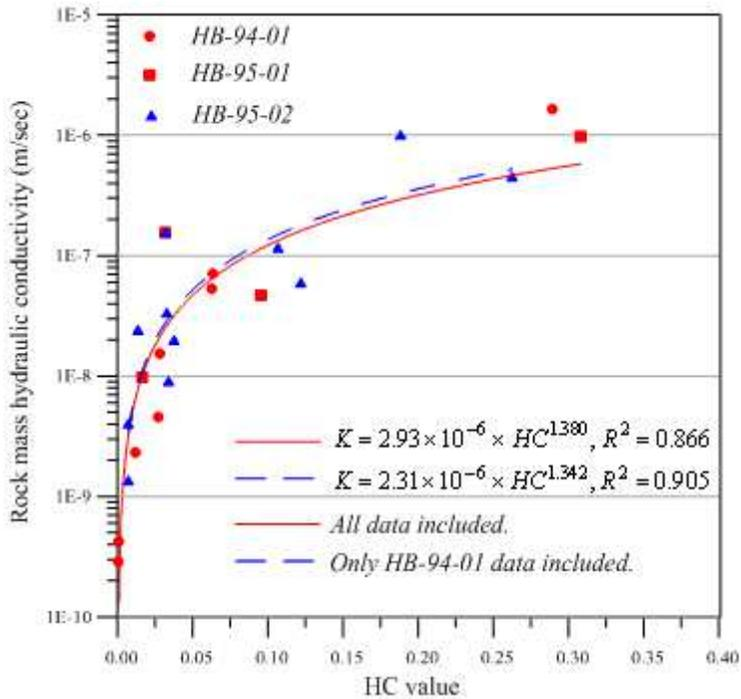
Fig. 6. Relationship between hydraulic conductivity and HC values
