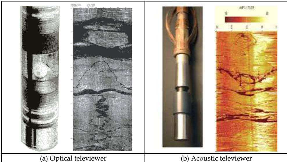
Fig. 8. The televiewer and scanned borehole images
