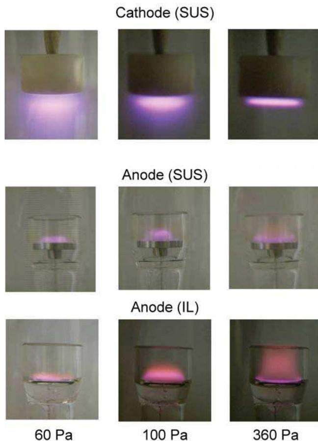
Fig. 4. Photos of the stable DC discharge plasma in B-mode in the regions below the cathode electrode and above the anode electrodes consisting of the SUS and the IL as a function of gas pressure  $P_{\text{gas}}$ .  $I_D = 1$  mA.
