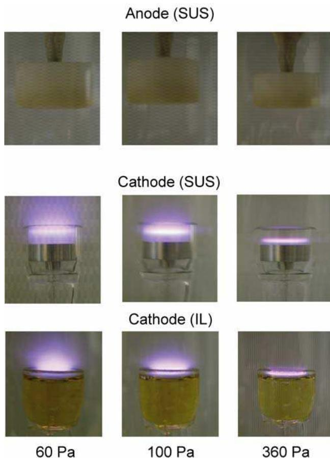
Fig. 3. Photos of the stable DC discharge plasma in A-mode in the regions below the anode electrode and above the cathode electrodes consisting of the SUS and the IL as a function of gas pressure  $P_{\text{gas}}$ .  $I_D = 1$  mA.
