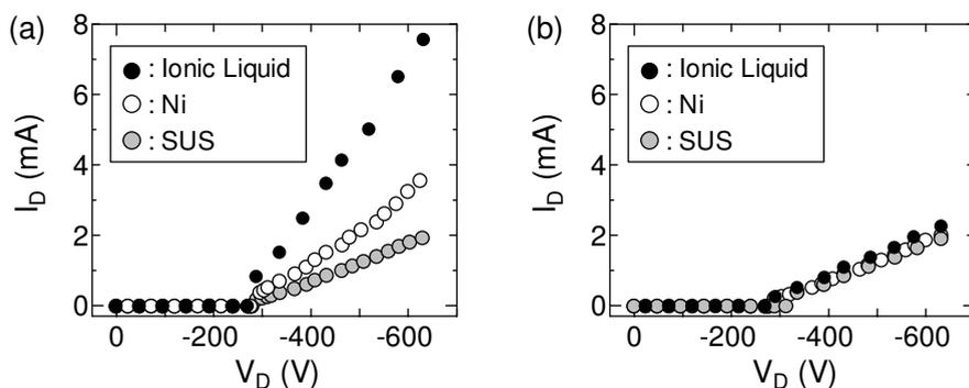
Fig. 7. Dependence of the discharge voltage  $V_D$  - current  $I_D$  characteristics on the materials of (a) the cathode electrode in A-mode and (b) the anode electrode in B-mode.  $P_{\text{gas}} = 40$  Pa. Ionic liquid is [BMI<sup>+</sup>][BF<sub>4</sub><sup>-</sup>].
