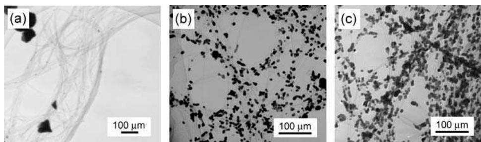
Fig. 15. TEM images of Au nanoparticles synthesized using the functionalized SWNTs, which are treated by the plasma irradiation in the ionic liquid for (a) 0 min, (b) 1 min, and (c) 10 min.  $P_{Ar} = 60$  Pa,  $I_D = 1$  mA.
