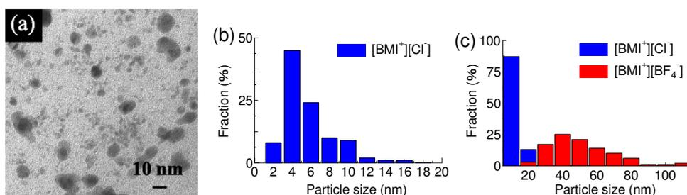
Fig. 13. (a) TEM images of the Au nanoparticles synthesized using the ionic liquid  $[\text{BMI}^+][\text{Cl}^-]$ .  $P_{\text{Ar}} = 60$  Pa,  $I_D = 1$  mA,  $t = 15$  min. (b) Particle size distribution of the Au nanoparticles synthesized in the ionic liquid  $[\text{BMI}^+][\text{Cl}^-]$  estimated by TEM image in Fig. 13(a). (c) Comparison of the particle size distributions between the cases of  $[\text{BMI}^+][\text{Cl}^-]$  and  $[\text{BMI}^+][\text{BF}_4^-]$ .
