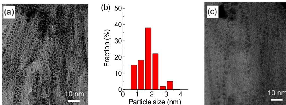
Fig. 14. TEM images of (a) Au and (c) Pd nanoparticles synthesized using the SWNTs as a template.  $P_{Ar} = 60$  Pa,  $I_D = 1$  mA,  $t = 15$  min. (b) Particle size distribution of Au nanoparticles onto the SWNTs estimated by TEM image in Fig. 14(a).
