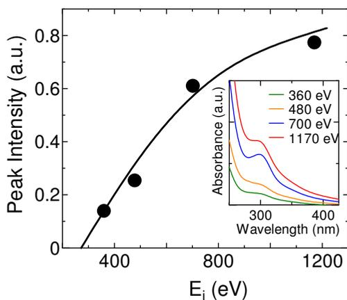
Fig. 9. Peak intensity of UV-Vis absorption spectra of the ionic liquid ( $[\text{BMI}^+][\text{BF}_4^-]$ ) at 297 nm as a function of the ion irradiation energy  $E_i$  in A-mode.  $I_D = 1$  mA,  $t = 2$  min. Inset is the absorption spectra with  $E_i$  as a parameter.
