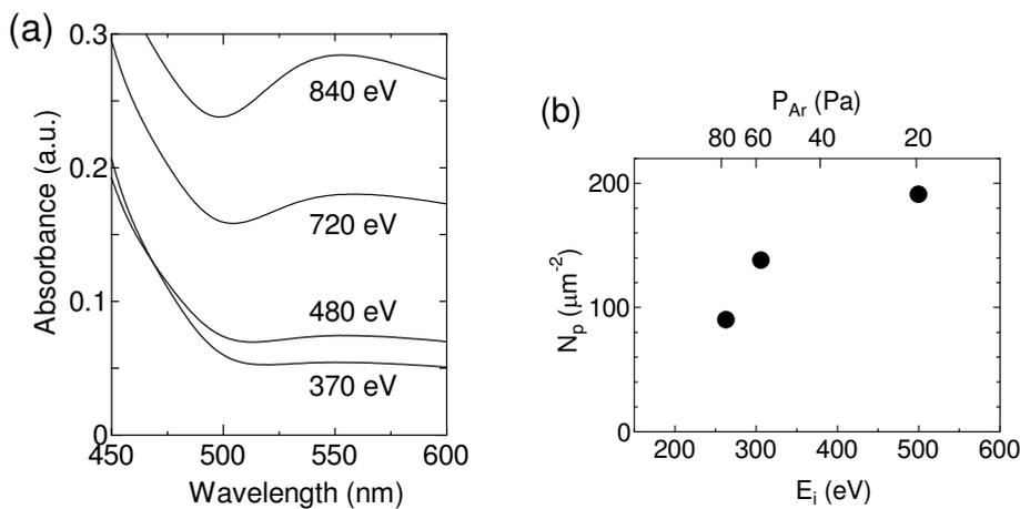
Fig. 12. (a) UV-vis absorption spectra of the Au nanoparticles produced by Ar plasmas as a function of ion irradiation energy  $E_i$  in A-mode.  $I_D = 1$  mA,  $t = 7$  min. (b) Spatially averaged number density  $N_p$  of the synthesized Au nanoparticles as a function of ion irradiation energy  $E_i$  in A-mode.  $I_D = 1$  mA,  $t = 40$  min.
