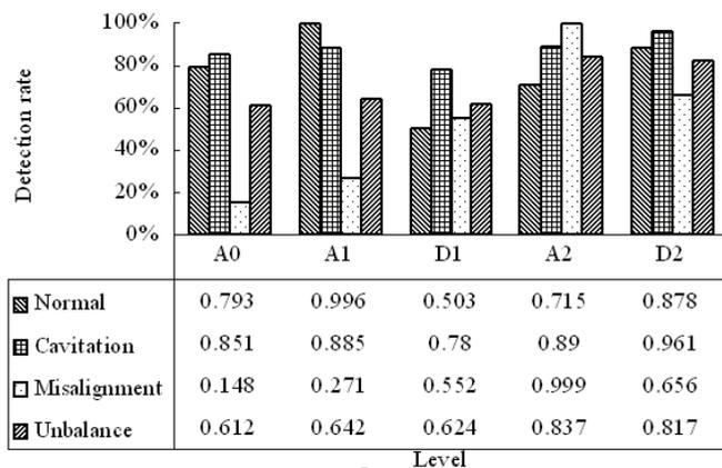
Fig. 2. Parts of detection rates in each state
