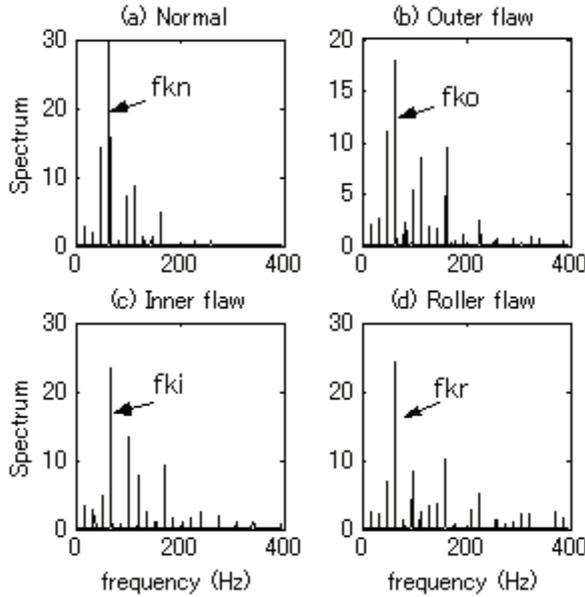
Fig. 11. Spectrums of enveloped diagnosis signal
