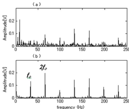
Fig. 7. Enveloped spectrums in outer-race flaw, (a) high-pass filtering, (b) adaptive filtering
