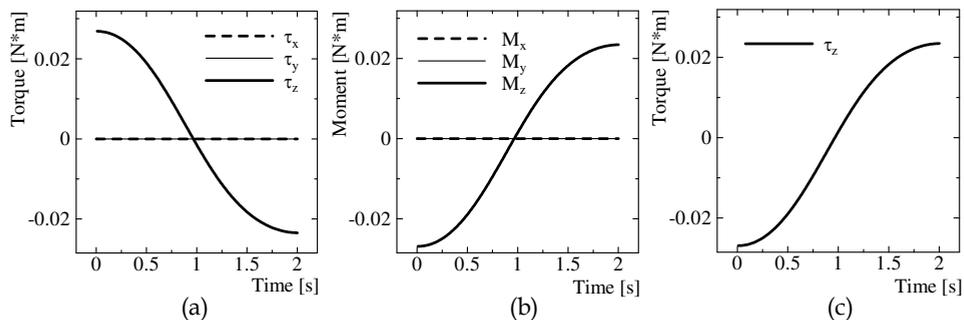
(a) Motion torques for driving a rotor
