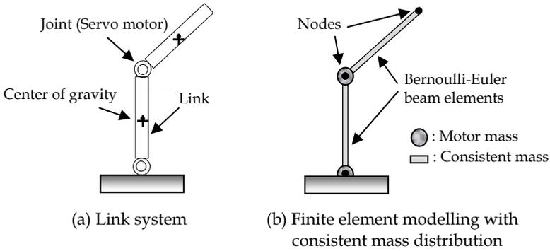
Fig. 1. Modelling of link systems using finite elements
