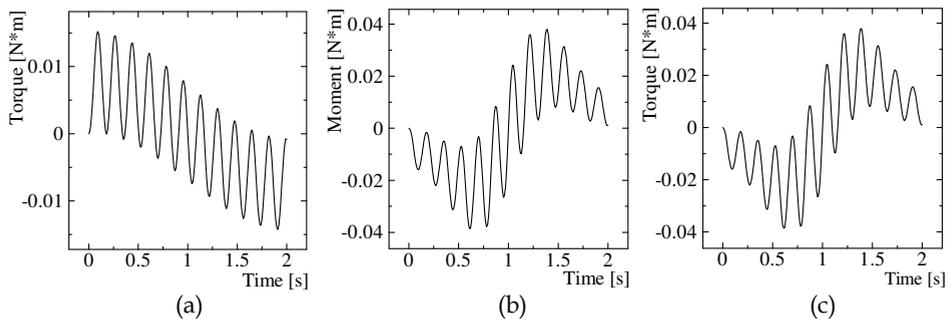
(a) Motion torque for driving the flexible link
