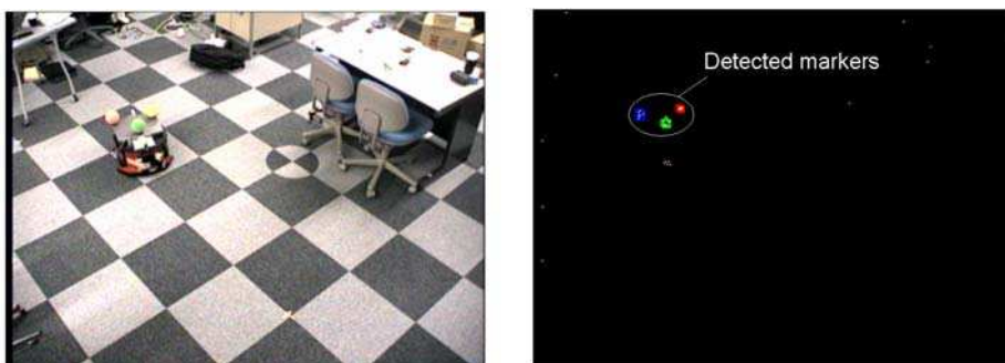
Fig. 6. Detection of color markers on a mobile robot using a camera DIND
