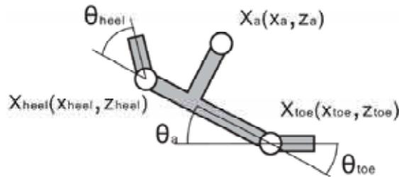
Fig. 14. Link vector configuration of the biped foot
