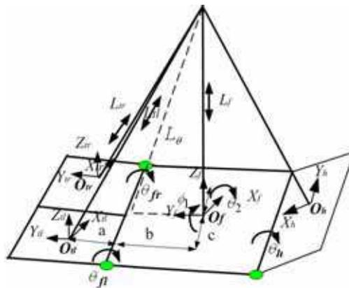
Fig. 9. The kinematic model of the foot mechanism
