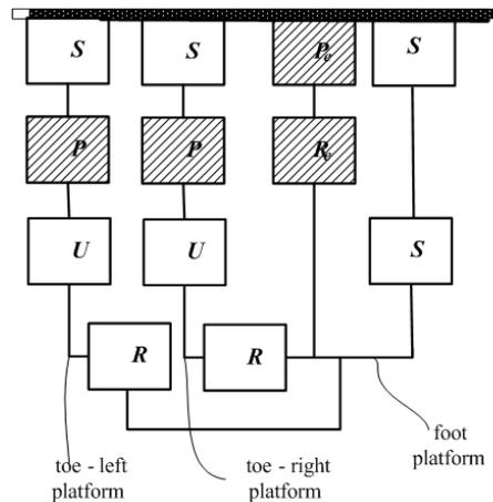
Fig. 4. The link-pair relationship diagram of the 4-dof mechanisms with three platforms
