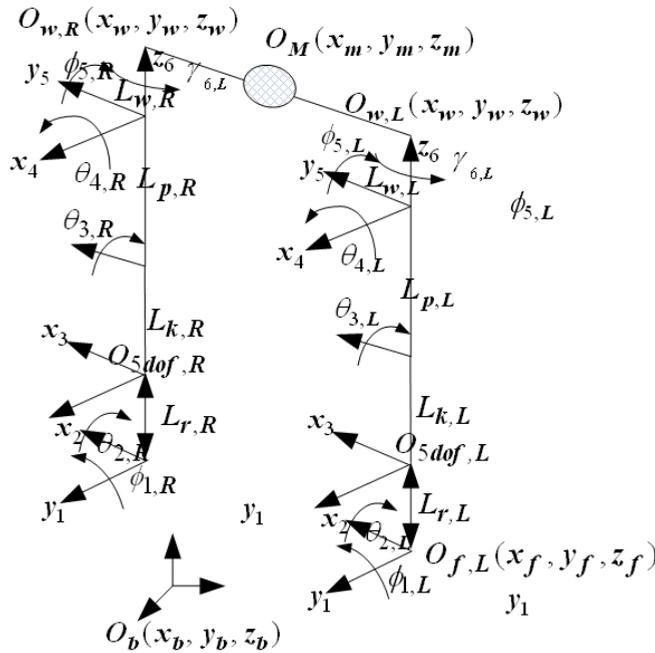
Fig. 8. Coordinate system of the biped robot
