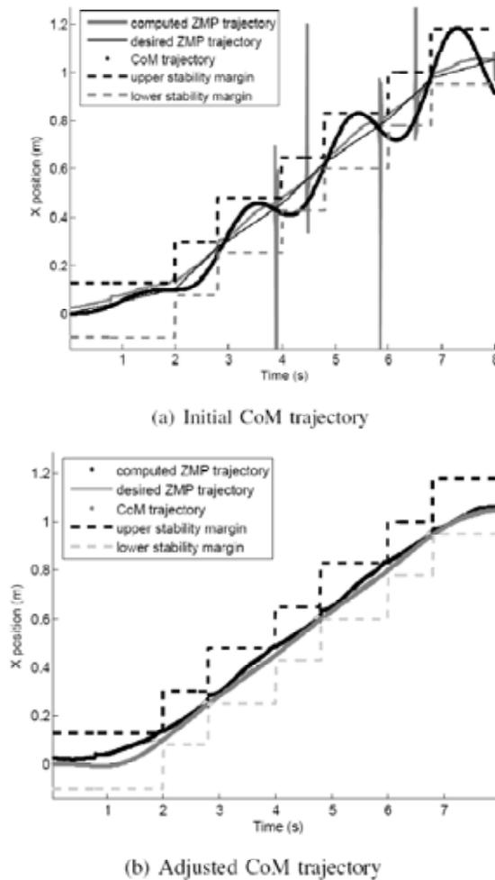
Fig. 16. Comparison between initial and adjusted CoM trajectories
