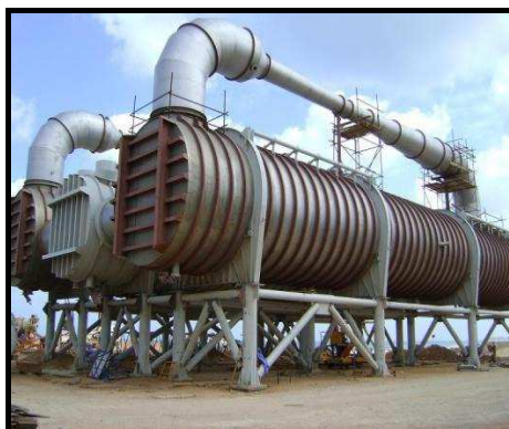
(a) Circular vessel evaporator.
