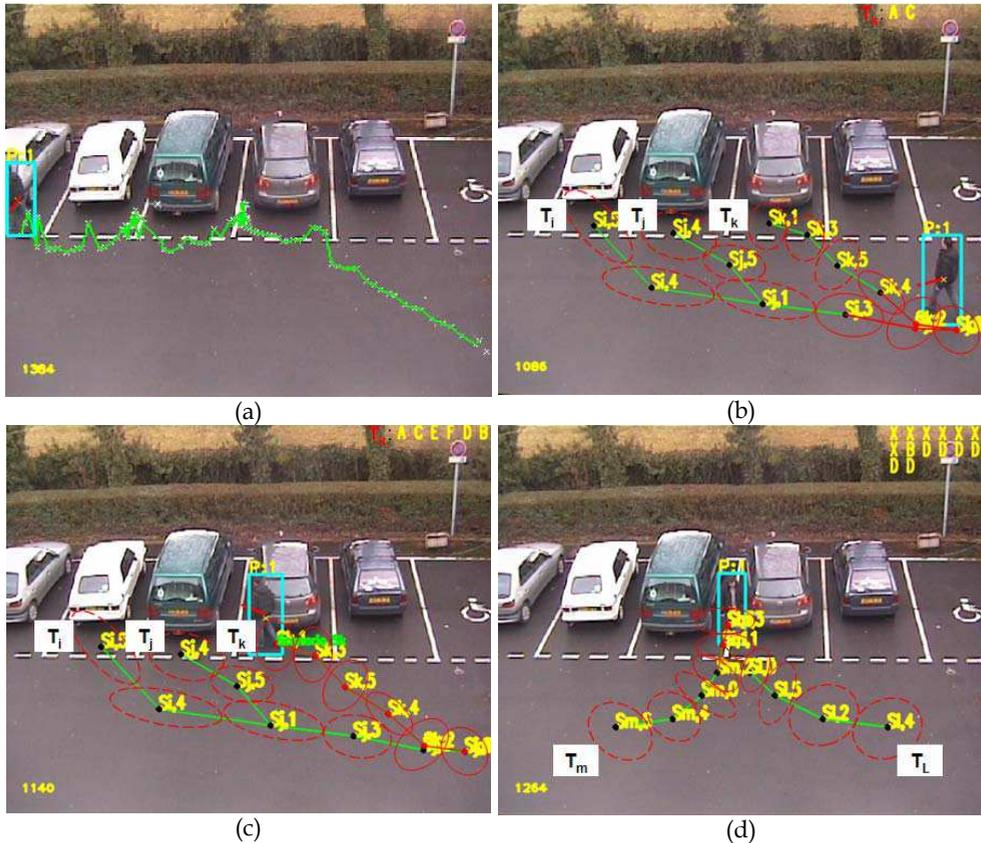
Fig. 10. (a) a global trajectory example; (b,c) : recognition of trajectories  $T_i, T_j, T_k$  linked with the 1st sub-scenario; (d) : recognition of trajectories  $T_m, T_l$  linked with the 2nd sub-scenario
