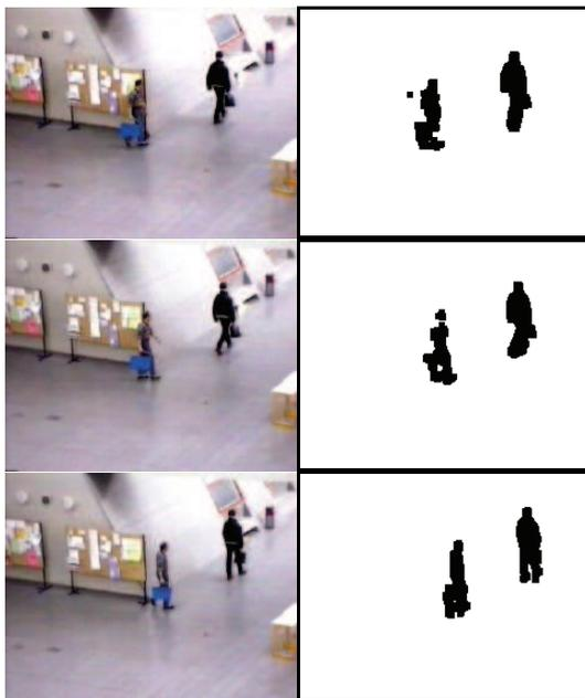
Fig. 1. Moving object segmentation, test images from the dataset PETS'2006, camera C3
