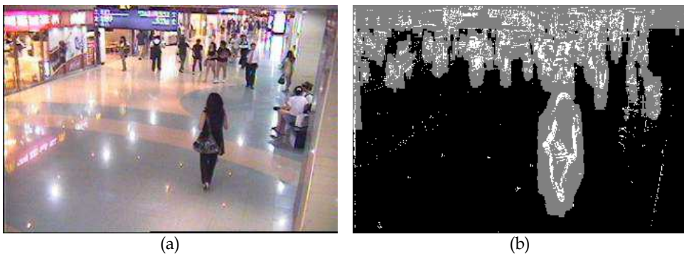
Fig. 5. Distinguishing static and non-static pixels: (a) input video frame; (b) black pixels and white pixels correspond to static and non-static pixels, respectively. Gray pixels are expanded from white pixels by morphological operations.
