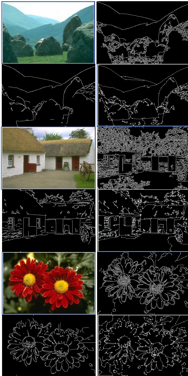
Fig. 7. For each example: a) original image; b) edge map detected by Canny edge detector; C) curves detected by Canny-based curve detection (Grigorescu et al., 2004); d) GET map detected by the color-based GET tracker.
