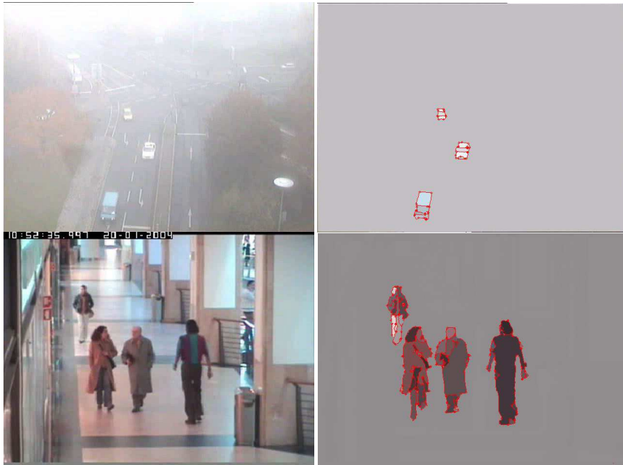
Fig. 9. Video surveillance system: GET maps and perceptual features of moving objects detected by the color-based tracker.
