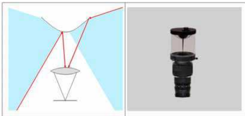
Fig. 3. Single mirror catadioptric optic. On the left the optic's schema, on the right a catadioptric lens.
