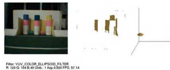
Fig. 3. Use of different bounding subspaces as color classes for classification of yellow in different color spaces. From left to right: Original image, Pixels from the original image classified as yellow, 3D representation of the color subspace. a) YUV Parallelepiped color class. b) RGB Cone color class. c) RGB Paraboloid color class. d) YUV Ellipsoid color class.
