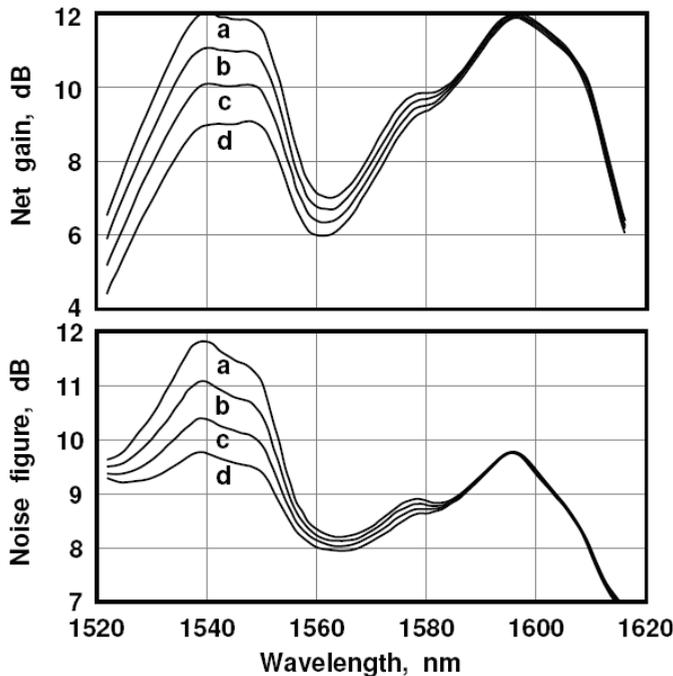
Fig. 14. Top: Gain variation with wavelength, Bottom: Noise figure variation with wavelength. Launched pump powers,  $P(\lambda_{p1})$ ,  $P(\lambda_{p2})$  in mW: (a) 716.3 and 227.8; (b) 642.0 and 241.0; (c) 569.5 and 255.1; (d) 496.5 and 271.8. Other amplifier characteristics are as in Fig. 12.
