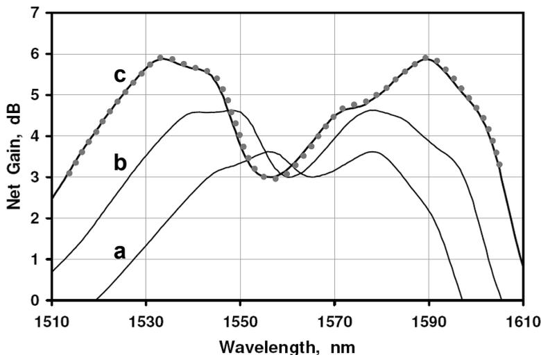
Fig. 17. Spectral gain variation with two pump wavelengths. Fibre length is 10 km and the pump loss coefficient  $\alpha_p$  is the average of  $\alpha(\lambda_{p1})$  and  $\alpha(\lambda_{p2})$ . Other data are in Table 2.
