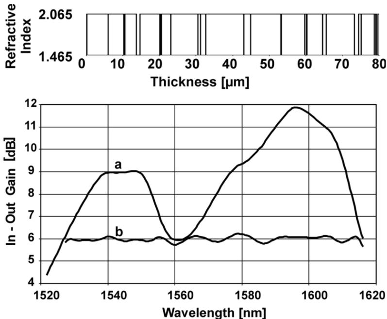
Fig. 16. Top: Thin film filter design (with 23 SiO<sub>2</sub> layers) to achieve spectral equalisation of the gain Curve d of Fig. 14. Bottom: The spectral gain variation before (Curve a) and after (Curve b) the filter is applied.
