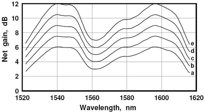
Fig. 12. Input-output gain as a function of wavelength for the following launched pump powers,  $P(\lambda_{p1})$ ,  $P(\lambda_{p2})$  in mW: (a) 281.7 and 120.5; (b) 356.3 and 142.0; (c) 448.5 and 166.1; (d) 565.4 and 194.1; (e) 716.3 and 227.8. The DCF length is 8 km.
