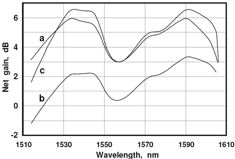
Fig. 4. Gain spectra for a dual-wavelength pumped DCF of length  $L = 10$  km. Curve a: small signal operation, 151 channels with -35 dBm/channel (but only 115 of them are plotted). Curves b and c: 115 channels spaced 100 GHz with -3 dBm/channel. The pump powers are stated in Table 1.
