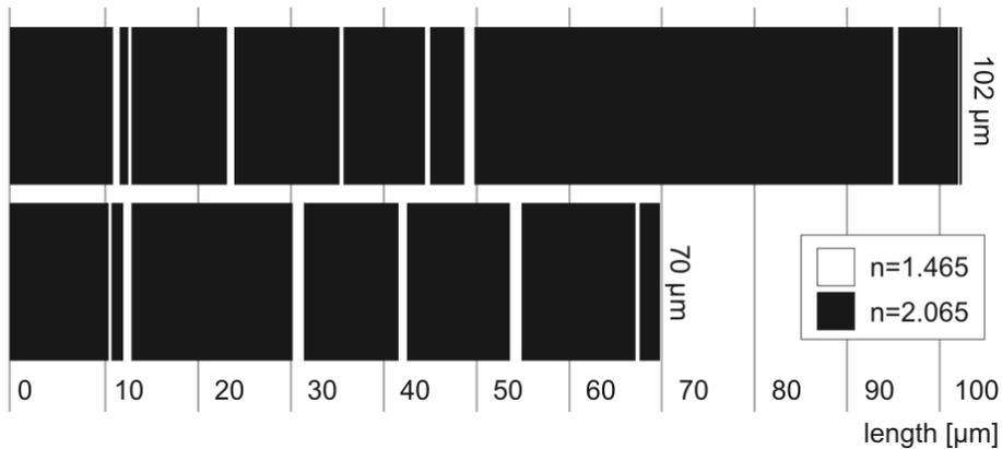
Fig. 6. Thin film structures formed from layers of  $\text{SiO}_2$  (refractive index 1.465) in  $\text{Ta}_2\text{O}_5$  (refractive index 2.065). Top: fifteen-layer filter to flatten Curve a in Fig. 4. Bottom: fourteen-layer filter to flatten Curve c in Fig. 4. The finer layers are not easily seen.
