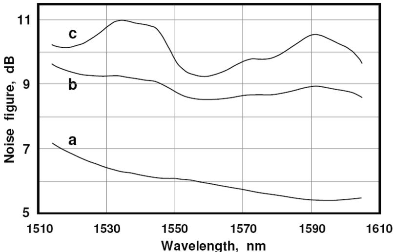
Fig. 5. Noise figure spectra for a dual-wavelength pumped DCF of length  $L = 10$  km. Curve a: small signal operation, 151 channels with -35 dBm/channel (but only 115 of them are plotted). Curves b and c: 115 channels spaced 100 GHz with -3 dBm/channel. The pump powers are stated in Table 1.
