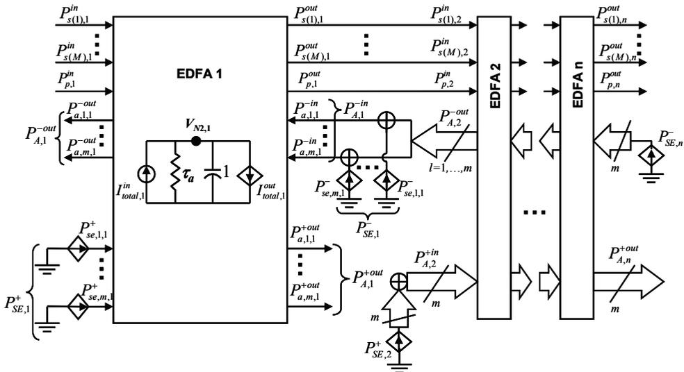
Fig. 1. Equivalent circuit model of EDFA including ASE
