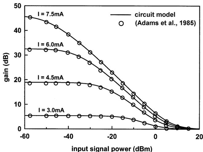
Fig. 9. Gain against input signal power for TW-SOA
