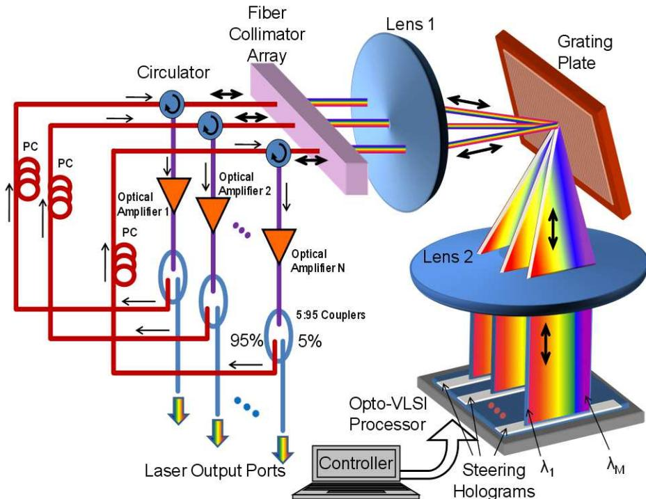
Fig. 9. The proposed multi-port tunable fiber laser structure.
