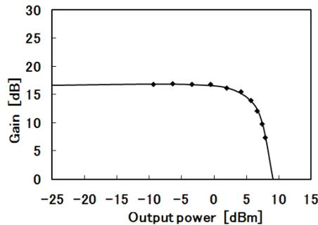
Fig. 11. Characteristic of saturation gain curve for NF-SOA.
