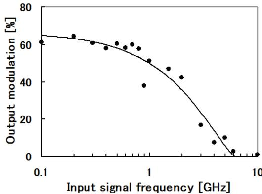
Fig. 19. Output modulation degree versus input signal frequency.
