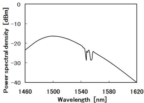
Fig. 12. Amplified spontaneous emission (ASE) spectrum for NF-SOA.
