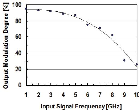
Fig. 23. Output modulation degree versus input signal frequency.
