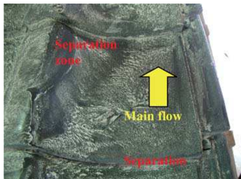
Fig. 9. Observation of the flow on the surface of the roof tile by the oil film method
