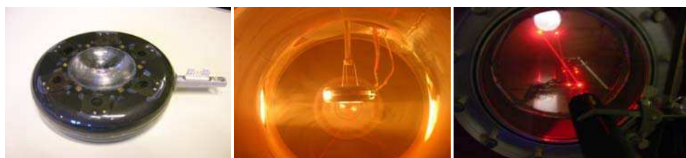
Fig. 8. Photographs of Laser Anemometers (acting also as suspended dust sensors), Left prototype time of flight instrument, Center the sensor during aerosol testing in an environmental wind tunnel, Right A commercial Laser Doppler Anemometer operating through an environmental wind tunnel access window, note the beams illuminating the suspended dust in the flow.
