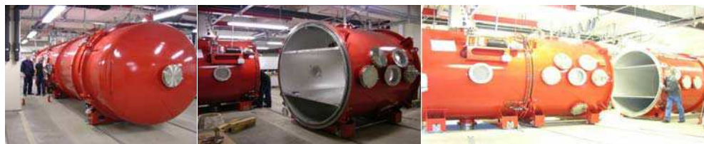
Fig. 4. Photographs of the (10m long) AWTS-II facility showing the mobile environmental chamber sections, the central test section can be removed laterally.
