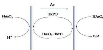
Fig. 9. Schematic representation of neutral As(III) with Cyanex 923
