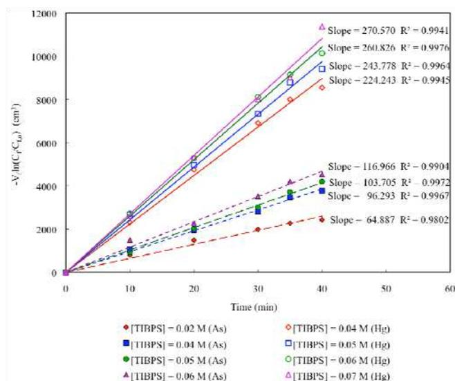
Fig. 14. Plot of  $-V_f \ln(C_f/C_{f,0})$  of arsenic and mercury ions in feed solution against time with different concentrations of Cyanex 471 mixed with 0.22 M Aliquat 336 for synergistic organic extractant
