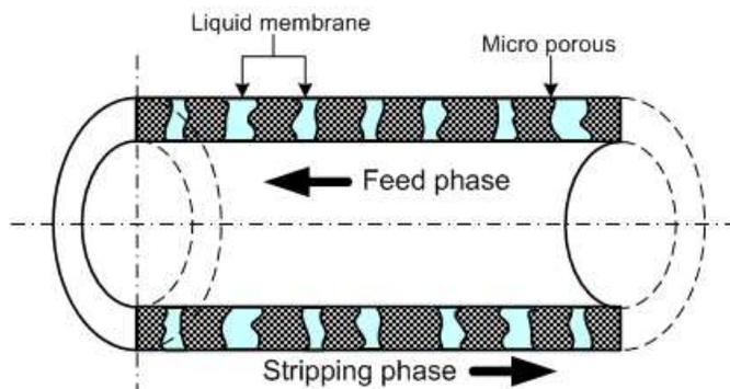
Fig. 2. The microporous hollow fiber liquid membrane
