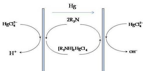
Fig. 10. Co-transport scheme of  $\text{HgCl}_4^{2-}$  by TOA extractant
