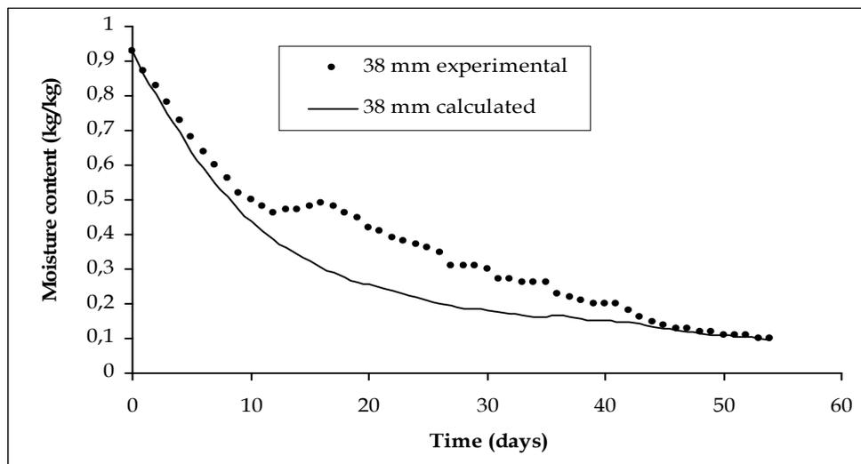
Fig. 5. Kiln drying curve of Chilean coigüe
