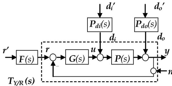
Fig. 2. Two degree of freedom MIMO control system
