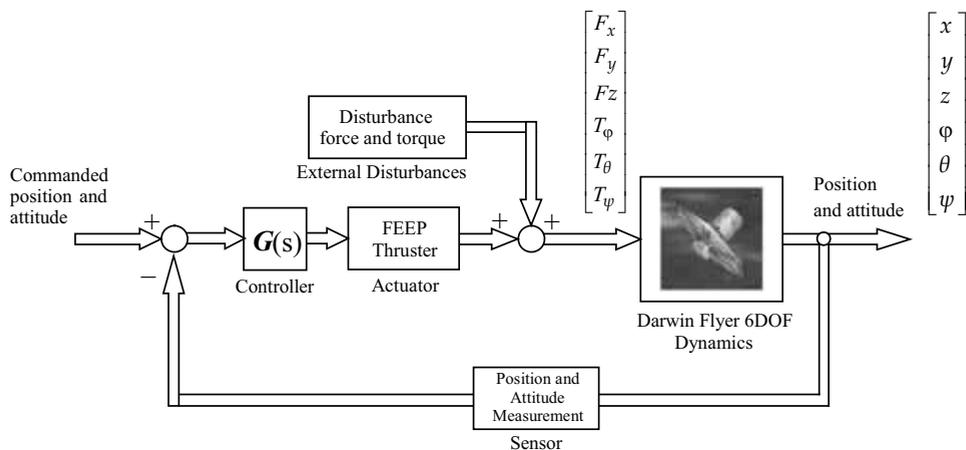
Fig. 10. ESA Telescope-type Spacecraft Simulator
