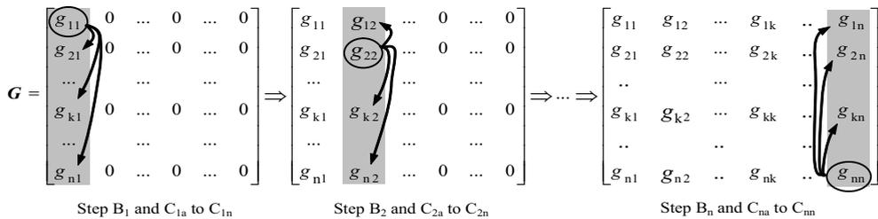
Fig. 3. Sequential steps for  $G(s)$  controller design
