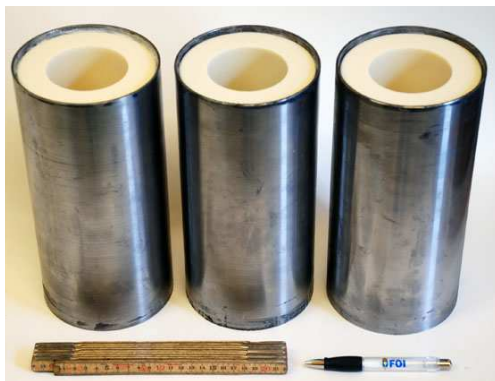
Fig. 9. Case bonded 3 kg ADN/GAP (70/30) grain cartridges for motor testing.
