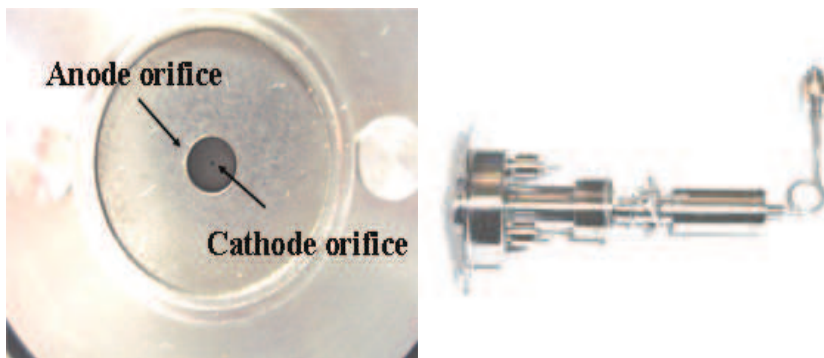
Fig. 6. T5 Hollow Cathode Thruster
