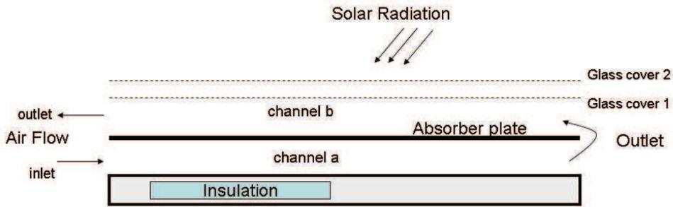
Fig. 4. Schematic view of double- pass solar air heater
