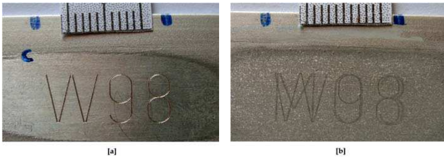
Fig. 2. a) Original engraved marks MO3 on Al (99% purity) surface were erased (hence not seen) and a new marks W98 were engraved over the erased area. b) The original marks MO3 were restored in the presence of the new marks W98. Note partial overlapping of the original digits "0" and "3" respectively with the new ones "9" and "8". Etching reagent: Alternating swabbing of 60% HCl and 40% NaOH. Etching time: 20 min.
