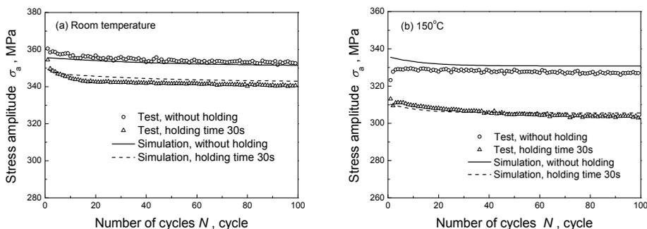
Fig. 13. Experimental and simulated results of responded stress amplitude vs. number of cycles for 6061-T6 aluminium alloy in the uniaxial symmetrical strain-controlled cyclic loading with strain amplitude of 0.6% and varied hold-time at peak and valley strains: (a) at room temperature; (b) at 150°C. (Originally from Ding et al. (2010))
