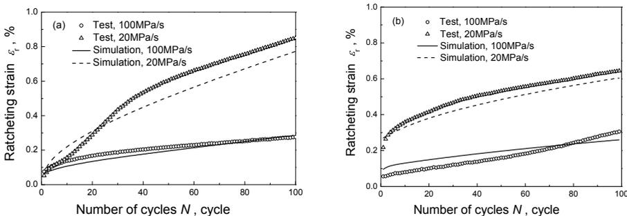
Fig. 16. Experimental and simulated results of time-dependent ratchetting for 6061-T6 aluminium alloy at two stress rates: (a)  $20 \pm 340$  MPa, at room temperature; (b)  $30 \pm 300$  MPa, at  $150^\circ\text{C}$ . (Originally from Ding et al. (2010))
