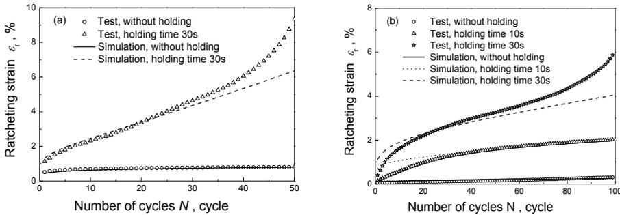
Fig. 17. Experimental and simulated results of time-dependent ratchetting of 6061-T6 aluminium alloy with different hold-times at peak stress (stress rate 100MPa·s<sup>-1</sup>): (a) 30±340MPa, at room temperature; (b) 30±300MPa, at 150°C. (Originally from Ding et al. (2010))
