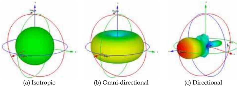
Fig. 2. Three dimensional radiation patterns
