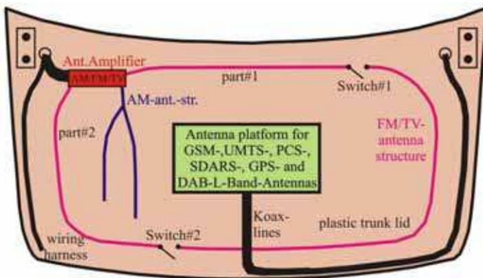
Fig. 22. Active antennas integrated into Plastic Trunk Lid
