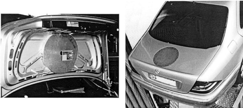
Fig. 18. Spiral antenna integrated into the trunk lid of a Mercedes Sedan
