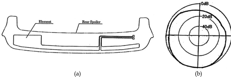
Fig. 14. Integrated antenna in spoiler
