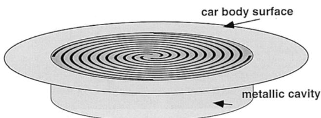
(a) Antenna design showing metallic cavity
