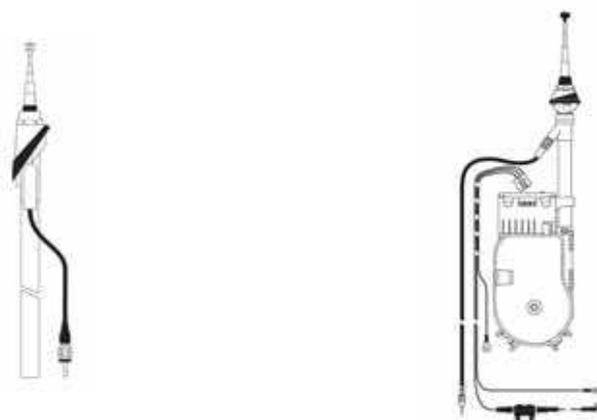
(a) Manually retractable mast antenna
