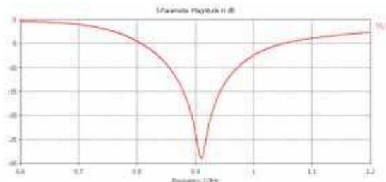
(a)  $|S_{11}|$  of a dipole Antenna
