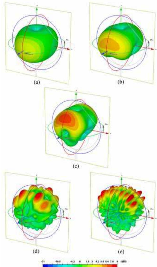
Fig. 21. Simulated 3D radiation patterns of the enlarged uniplanar CPW fed PICA. (a) 850 MHz, Max gain is 3.9 dBi (b) 1.575 GHz, Max gain is 5.7 dBi (c) 2.4 GHz, Max gain is 8.1 dBi (d) 5.9 GHz, Max gain is 9.6 dBi (e) 9.5 GHz, Max gain is 11 dBi
