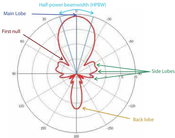
Fig. 3. A sample two dimensional radiation pattern
