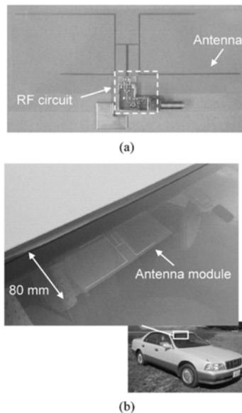
Fig. 12. Digital TV Antenna attached to vehicle glass
