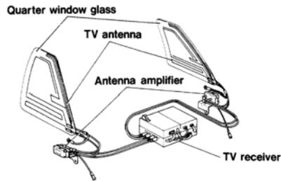
Fig. 11. Analogue TV Antenna system in rear quarter glass
