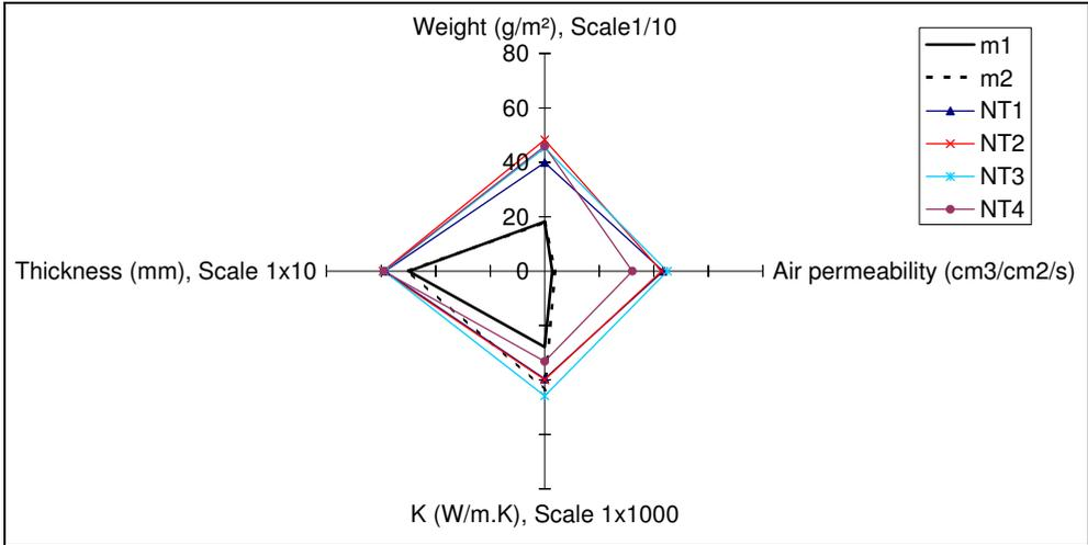
Fig. 22. Physical characteristics of the tested monolayer samples
