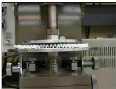
Fig. 20. Customization of the KES-FB3 compression tester
