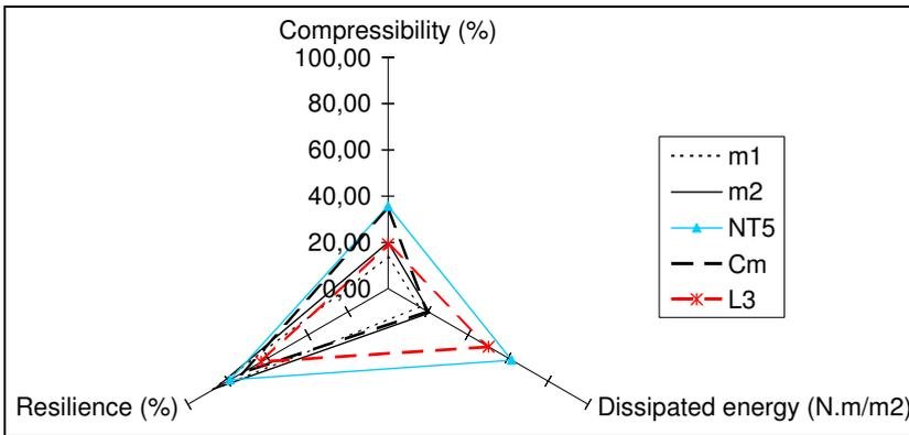
Fig. 31. Compressional characteristics of the tested samples
