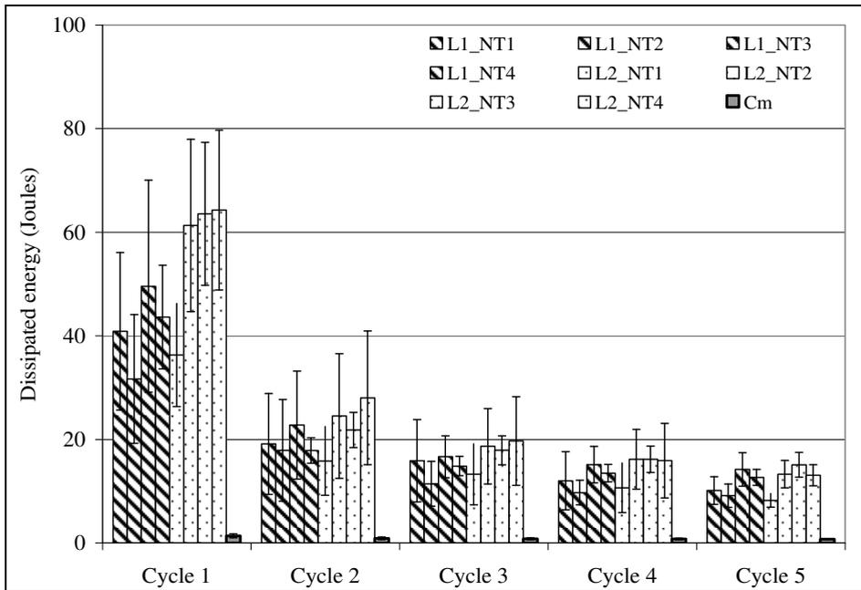
Fig. 29. Dissipated energy of the tested multilayer samples
