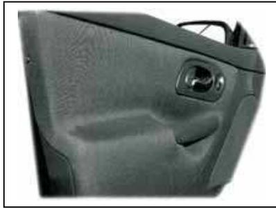
Fig. 2. Example of an integral door panel
