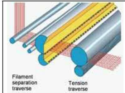
Fig. 13. The defibering principle
