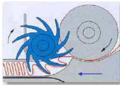
Fig. 9. The Santex WAVEMAKER® process
