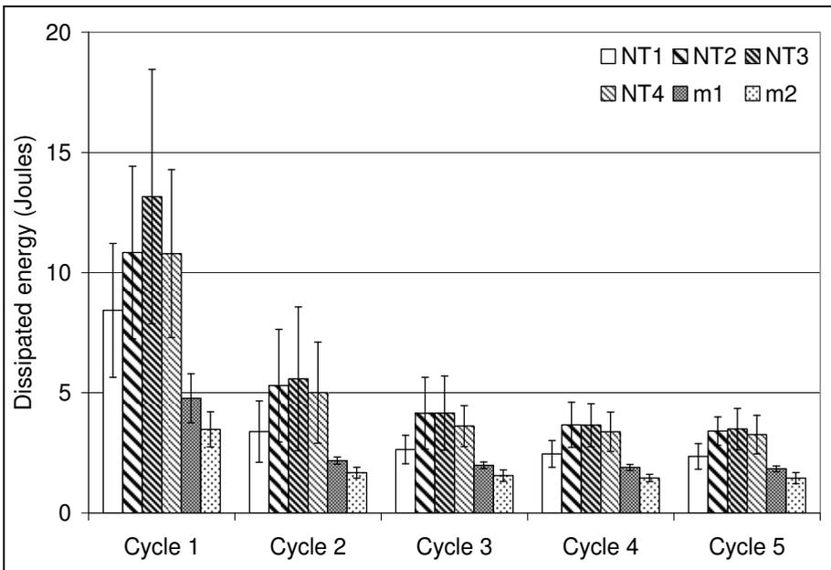
Fig. 27. Dissipated energy of the tested monolayer samples
