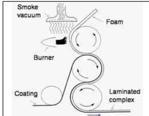
Fig. 4. The flame lamination process
