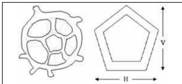
Fig. 17. Geometrical modelling of the PU foam
