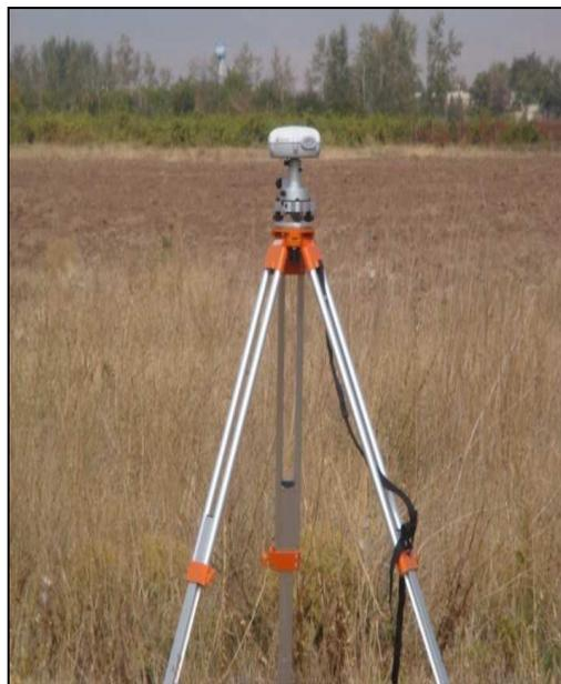
Fig. 6. A static GPS receiver.
