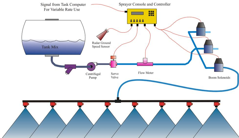
Fig. 1. A flow-based control system (adapted from Humburg [7]).
