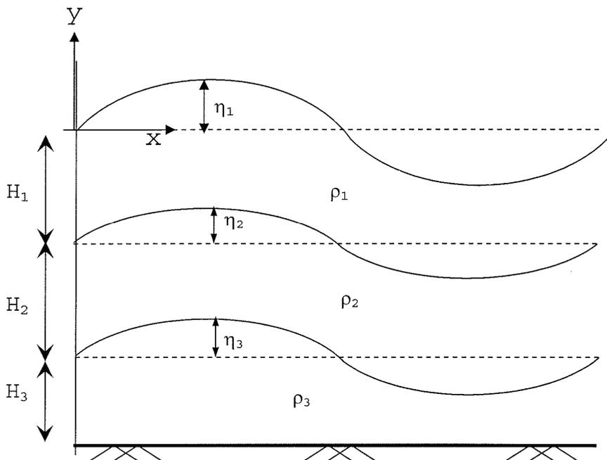
Fig. 1. Schematic diagram of three layer profile
