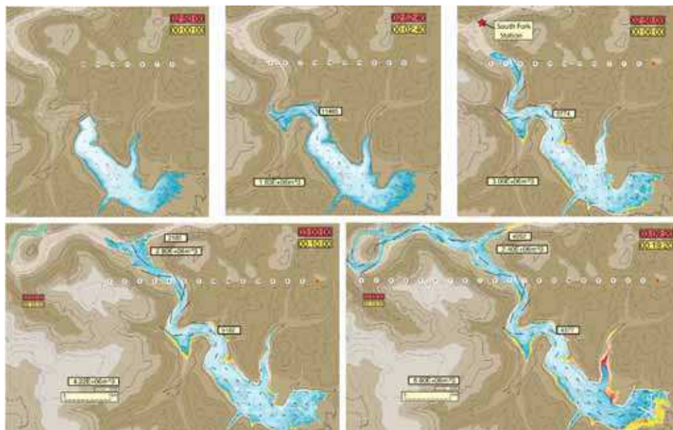
Fig. 6. Snapshots of the early phase of the flood simulation. The yellow backed clock gives elapsed time T = 00:00, 02:40, 06:00, 10:00 and 00:19:20 . The red backed clock gives clock time T = 2:50, 2:52, 2:56, 3:00 and 3:19 PM. Note up-river counter flow at the junction of the South Fork and Little Conemaugh Rivers (Panel D) and the floodwater cutting across the oxbow in front of the Viaduct (Panel E). (Movie at http:// es.ucsc.edu/ ~ward/ jtown-lake-close-s.mov ).
