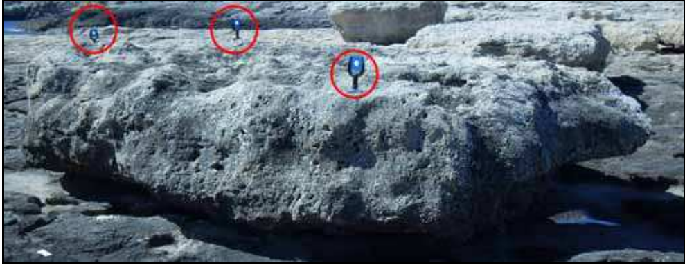
Fig. 5. Megaboulder scanned on the coastal area of Augusta (Southern Italy). Red circles highlighted the rectangular targets used to co-registrate all the TLS scan.
