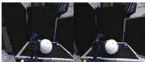
Fig. 24. a) Points over the sphere as seen by the robot "Geometer". b) Guiding spheres for the arm's motion.
