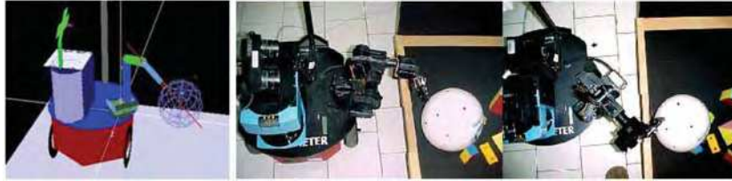
Fig. 25. a) Simulation of the motion over a sphere. b) and c) Two of the images in the sequence of the real experiment.
