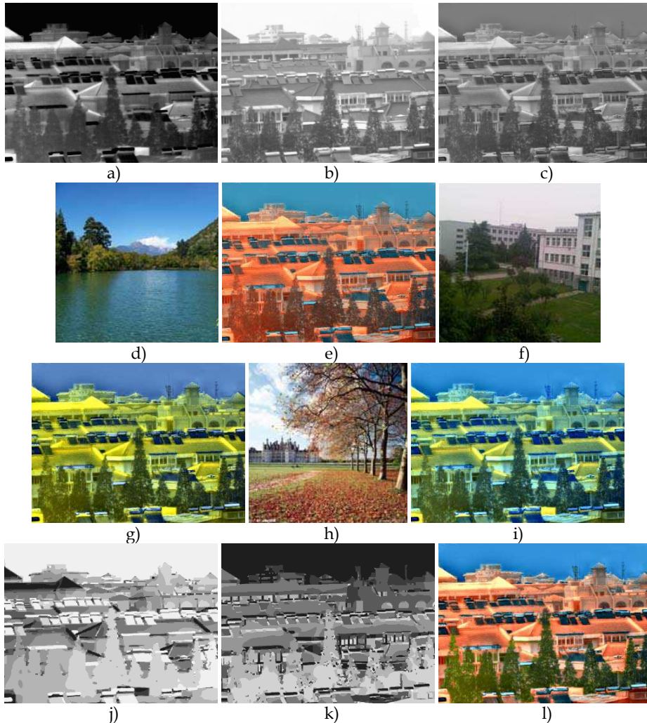
Fig. 7. Source images, reference images and fused results with different methods. (a) infrared image, (b) visible light image, (c) fusion image using gradient pyramid method, (e), (g) and (i) fusion images with global-coloring method separately using (d), (f) and (h) as reference image, (j) region map of the infrared image, (k) region map of the visible light image, (l) fused image with the region-based coloring fusion method using (d), (f) and (h) as reference images
