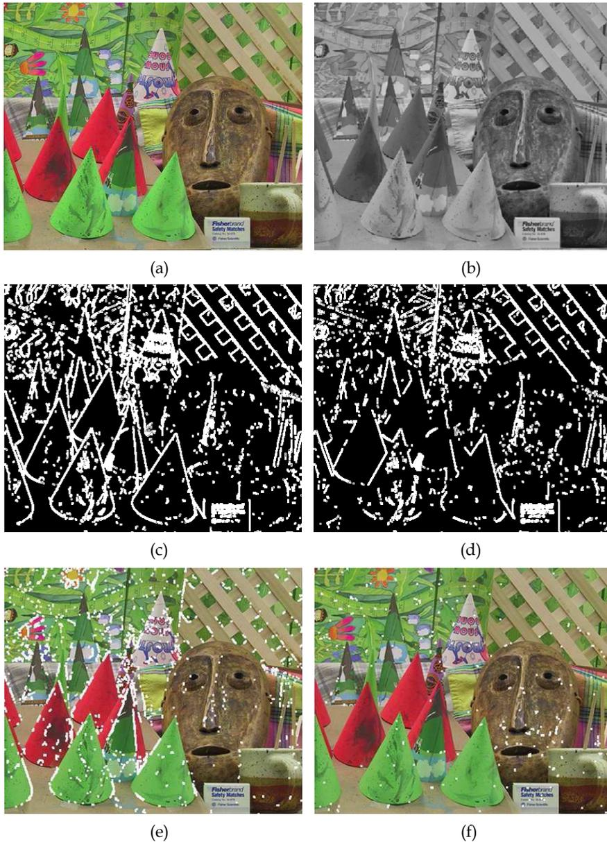
Fig. 7. Experimental results of color edges segmentation and gray level segmentation of Cones image of Middlebury database Scharstein & Szeliski (2002). (a) Color image. (b) The corresponding gray level image of (a). (c) Color-declivity image. (d) Declivity image. (e) Edge points extracted in color image but not in gray level image superimposed in white on color images. (f) Edge points extracted in gray level image but not in color image superimposed in white on color images.
