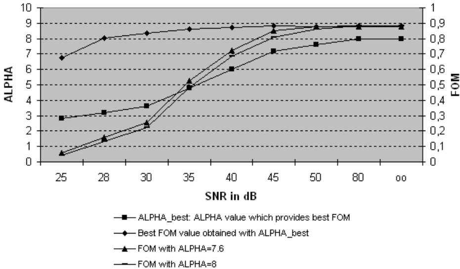
Fig. 3. Three Pratt’s figures-of-merit (FOM) computed with different value of  $\alpha$ ; and obtained from Lena image in which gaussian noise of different amplitude has been added  $SNR \in [25, \infty]$  dB.
