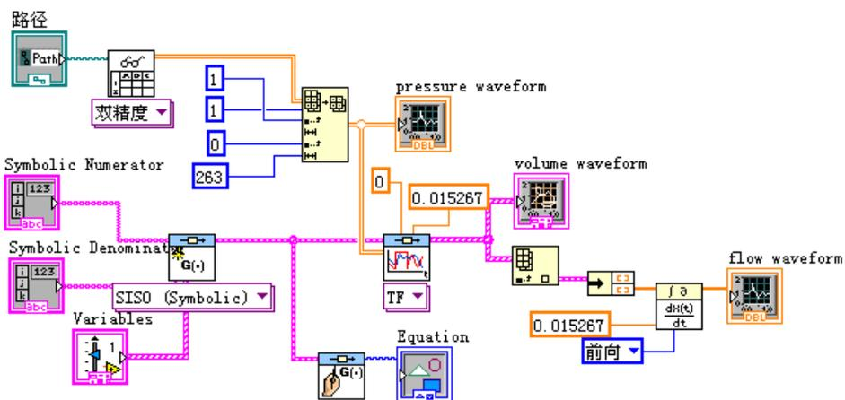
Fig. 8. Block diagram of respiratory simulation using transfer
