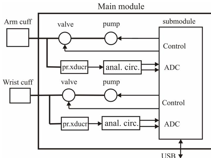
Fig. 3. Block diagram of the dual cuff system.
