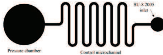
Fig. 11. Layout SU-8 mask for a pressurized chamber.
