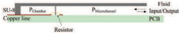
Fig. 16. Cross-section view of the 2D micro impulsion device. Pressure in the chamber is regulated through a PCB orifice.
