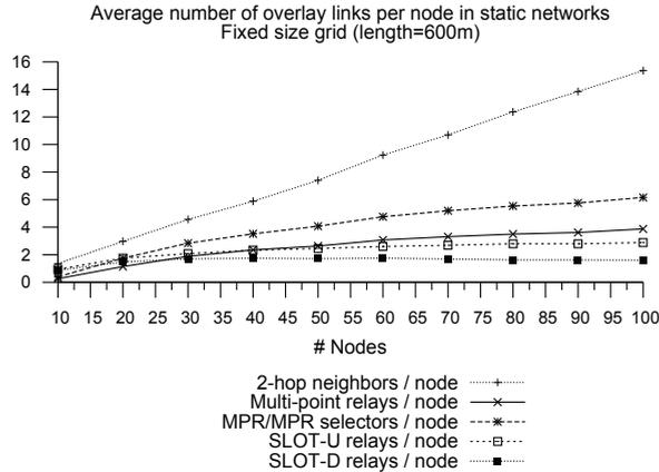
Fig. 12. Density of MPR and SLOT overlays in static networks. The SLOD-D simulations are computed with the quantized cost:  $cost(\overline{xy}) = \lceil K \frac{d(\overline{xy})}{r} \rceil$ , with  $K = 10$  and  $d(\overline{xy})$  being the Euclidean distance between  $x$  and  $y$ .
