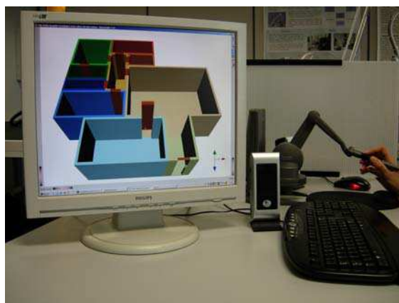
Fig. 2. The hapto-acoustic version of the World in Miniature metaphor used to navigate VE. The user pilots the avatar through the haptic stylus of a PHANToM Desktop
