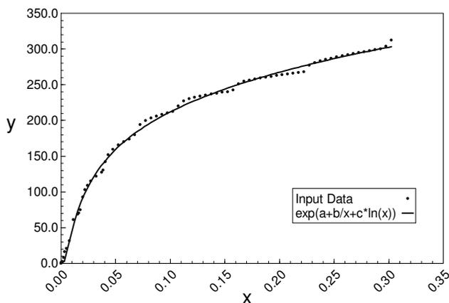
Fig. 9. Exponential adjustment of the Load-displacement curve in zone (I+II) until  $d=0.3$  mm. Moreover, it has been carried out sensitivity analyses within a  $\pm 10\%$  variation of the factors a, b, c of the exponential law, in order to analyse their effect on the load-displacement curve. These analyses show that the influence of the function a on the exponential law is enormous, the influence of c is notable and the influence of b is not important.
