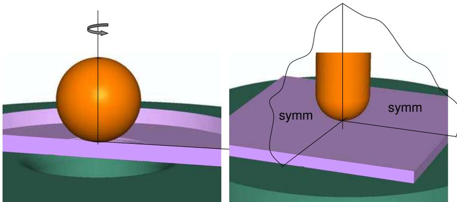
Fig. 4. Axisymmetric and Three-dimensional models used for the simulation of the SPT
