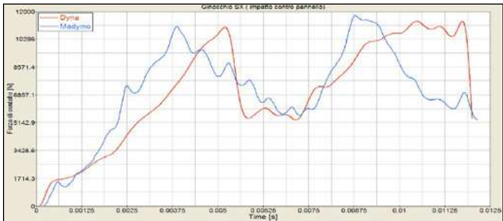
Fig. 26. Comparison between contact forces in Dyna-Madymo in the area of the SX knee
