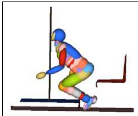
Fig. 24. 235 ms: the neck reaches the critical position: this is the maximum deflection
