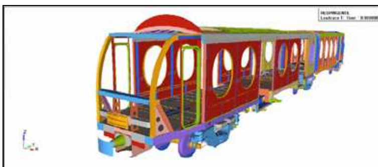
Fig. 21. The FEM model of a train coach
