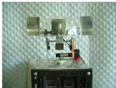
Figure 3. Front view of the robot with pinnae
