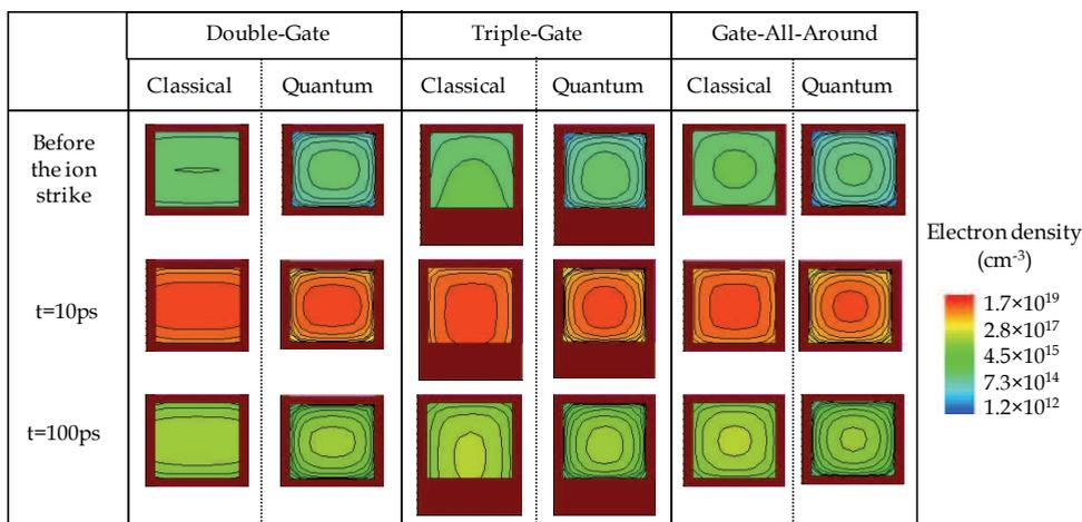
Fig. 6. Classical and quantum electron density (expressed in  $\text{cm}^{-3}$ ) in a vertical cross-section ( $y$ - $z$  plane) in the middle of the channel of 32 nm Double-Gate, Triple-Gate and Gate-All-Around at different times before and after the ion strike. The devices are biased in the off-state at  $V_G=0$  V and  $V_D=0.8$  V. The brown regions represent the gate oxide (in Double-Gate and Gate-All-Around devices) and the gate and buried oxide in Triple-Gate devices
