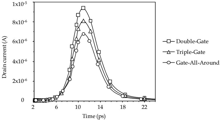
Fig. 7. Drain current transients induced by an ion strike vertically (y direction) in the middle of the Silicon film (classical simulation). The ion track generation has a Gaussian shape versus time (characteristic time of 2 ps), centred at 10 ps and a LET=1 MeV/(mg/cm<sup>2</sup>). The simulated devices are 32 nm gate length MOSFETs. All devices are off-state biased ( $V_G=0$  V,  $V_D=0.8$  V)
