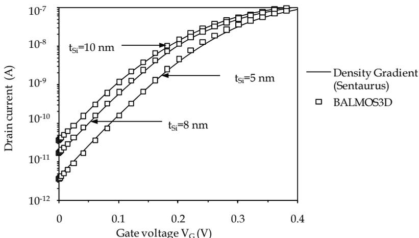
Fig. 3. Calibration of the Density-Gradient model (Sentaurus, 2009) on BALMOS3D. The simulated devices are 32 nm gate length Double-Gate MOSFETs with three Silicon thicknesses ( $t_{Si}=10$  nm, 8 nm and 5 nm). For better illustration, the figure only shows the subthreshold region of the drain current characteristics.  $V_D=0.8$  V
