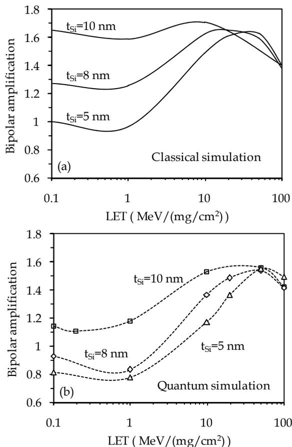
Fig. 10. Bipolar gain variation when reducing the Silicon film thickness in Gate-All-Around MOSFET with 32 nm gate length (the gate width is  $W=10$  nm): (a) classical simulation; (b) quantum simulation. The transistors are biased in the off-state at  $V_G=0$  V and  $V_D=0.8$  V
