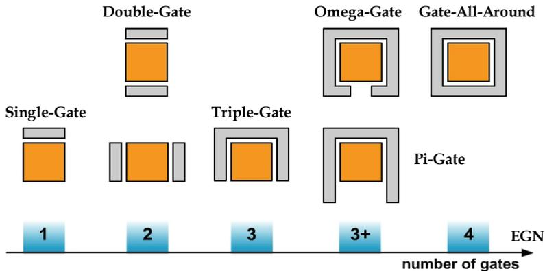
Fig. 1. Schematic cross-sections of the Multiple-Gate devices classified as a function of the "Equivalent Number of Gates" (EGN)
