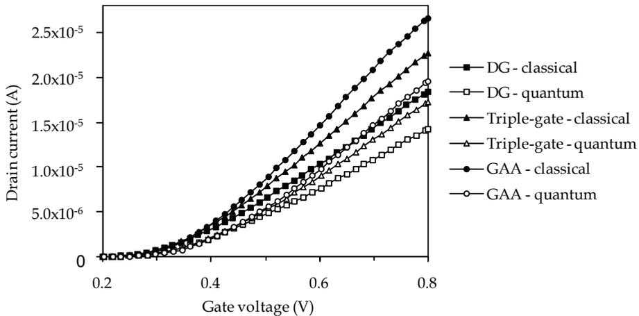
Fig. 5. Drain current  $I_D(V_G)$  characteristics in classical and quantum-mechanical cases for 32 nm Double-Gate, Triple-gate,  $\Omega$ -Gate and Gate-All-Around architectures ( $V_D=0.8$  V). The quantum drain current was simulated using the Density-Gradient model calibrated on BALMOS3D numerical results
