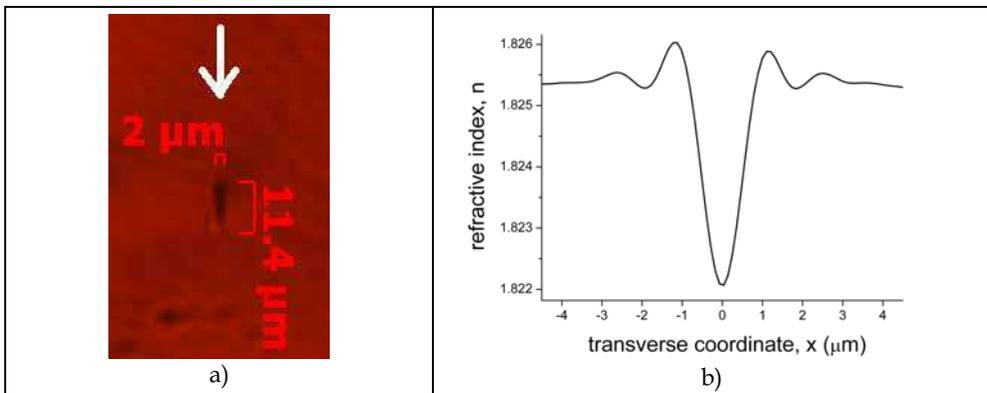
Fig. 17. a) Microscopic end view of a track inscribed in YAG:Nd(0.3%) crystal at a depth of 60  $\mu\text{m}$ . b) Refractive index profile of the same track. The arrow indicates the direction of the femtosecond beam and of observation when index profile was measured.
