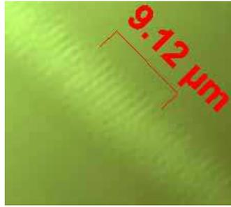
Fig. 12. Self-organised gratings inscribed in YAG:Cr<sup>4+</sup> crystal at wavelength of 400 nm with slow moving ( $V < 0.015$  mm/c).
