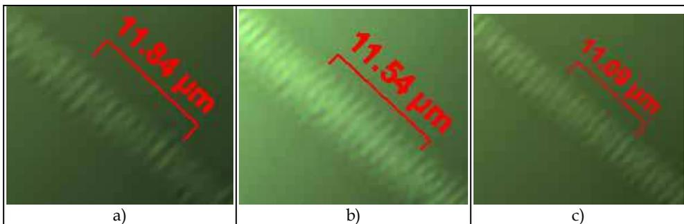
Fig. 13. Gratings inscribed in YAG:Cr<sup>4+</sup> crystal at wavelength of 400 nm by AOM modulation technique with beam of an elliptical cross-section;  $E_{in} = 0.56$   $\mu$ J:
