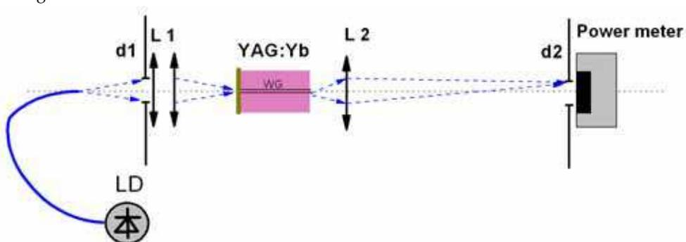
Fig. 10. Experimental setup for pump light attenuation measurements.
