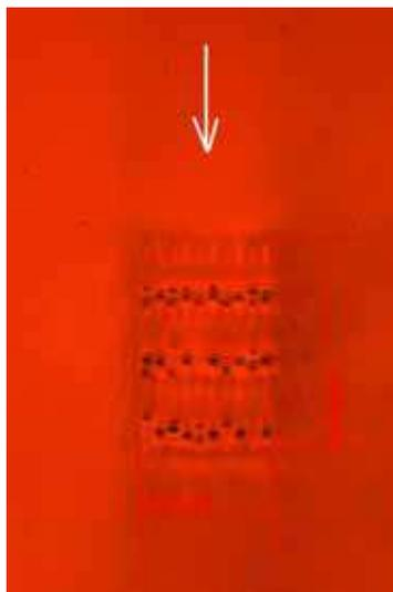
Fig. 2. End view of a waveguide written by Ti-Sapphire oscillator operating at 11-MHz rep rate. The arrow indicates direction of the femtosecond beam.
