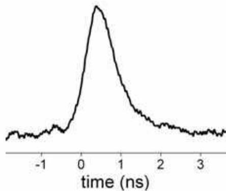
Fig. 23. Oscilloscope trace of a Q-switch pulse.
