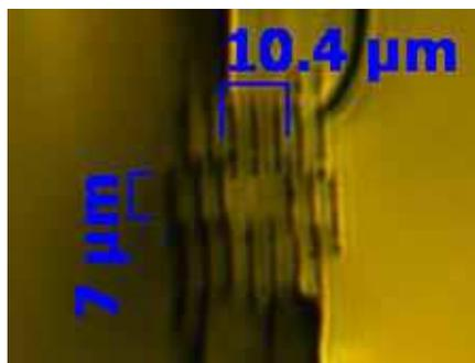
Fig. 6. End view of a depressed cladding waveguide inscribed in YAG:Cr<sup>4+</sup>
