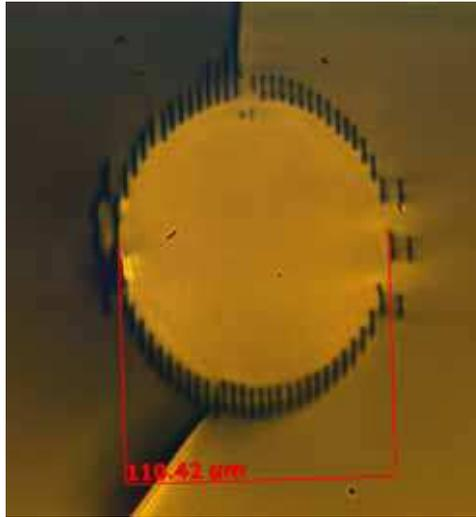
Fig. 7. End view of a depressed cladding multimode waveguide inscribed in diffusion bonded YAG:Nd/YAG:Cr<sup>4+</sup> crystal. The refractive index is lowered by nearly  $3 \times 10^{-3}$  in each track compared to the unperturbed value in the bulk of crystal.
