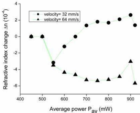
Fig. 16. Dependencies of PRICE and track height in YAG:Cr<sup>4+</sup> crystal upon average input power. 11 MHz rep rate femtosecond laser.
