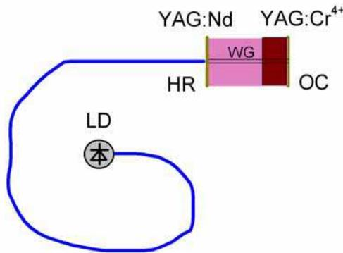
Fig. 21. Scheme of laser setup.
