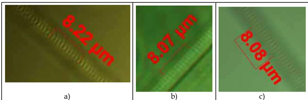
Fig. 11. Gratings inscribed in YAG:Cr<sup>4+</sup> crystal at wavelength of 800 nm with point-by-point technique (a,b) and AOM modulation (c):
