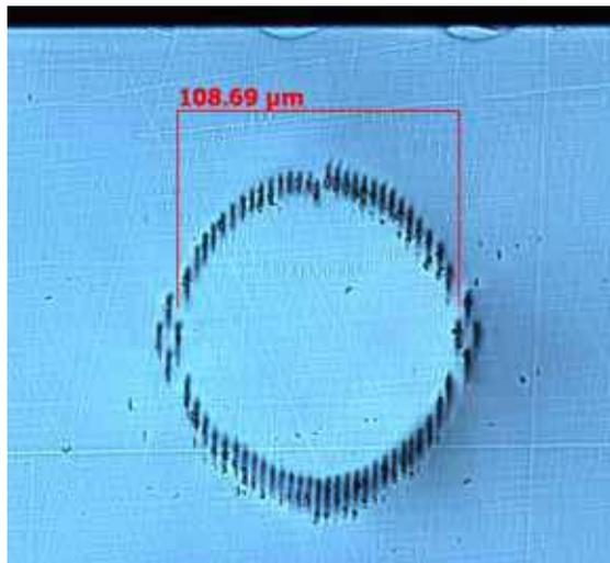
Fig. 8. End view of a depressed cladding waveguide inscribed in YAG:Yb<sup>3+</sup>
