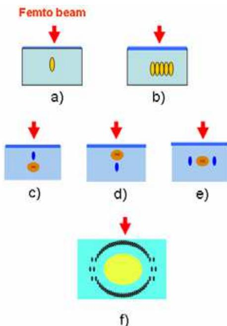
Fig. 1. Architectures of femtosecond written waveguides. Direct writing of a core: a) a single track, b) a multiple track core. Stress induced waveguides: c) and d) a waveguide is below and above the track, e) waveguide is in between two tracks. f) A micro-structured depressed cladding waveguide.
