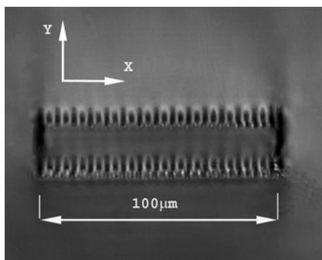
Fig. 5. End view of a depressed cladding waveguide inscribed in YAG:Nd<sup>3+</sup>.
