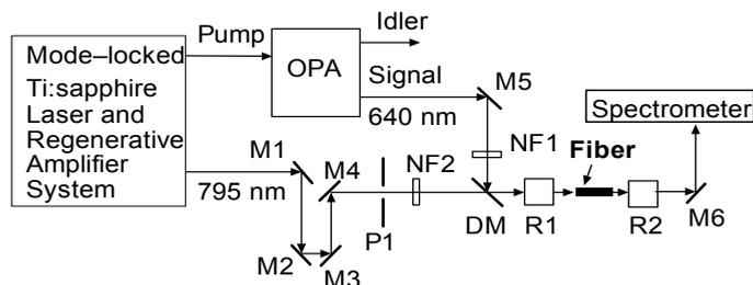
Fig. 10. Layout of the experimental setup. (Xu et al., 1999) M, silver-coated plane mirrors; R1 and R2, reflective objectives (36x); DM, dichroic mirror; NF1 and NF2, valuable optical attenuators; OPA, optical parametric amplifier.
