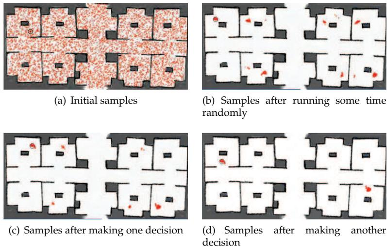
Fig. 8. Active localization of a single robot
