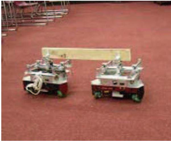
Fig. 5. Omni-wheeled robots utilized for experimentation
