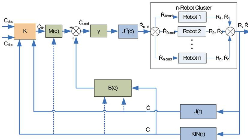
Fig. 3. Model-based kinematic cluster space control architecture for a mobile *n*-robot system. Desired control velocities are computed in cluster space and a partitioned control architecture decouples the system. The inverse Jacobian matrix converts the resulting cluster space velocities to robot space velocities that are then applied to the system. Robot sensor information is converted to cluster space through the Jacobian and kinematic relationships.
