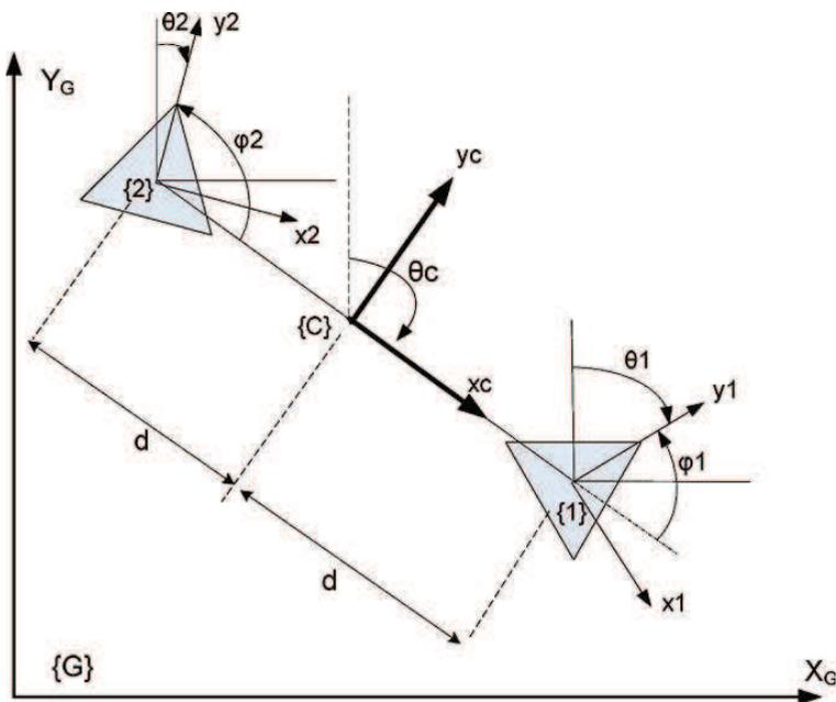
Fig. 4. Reference frame definition placing the cluster center at the center of the two robots
